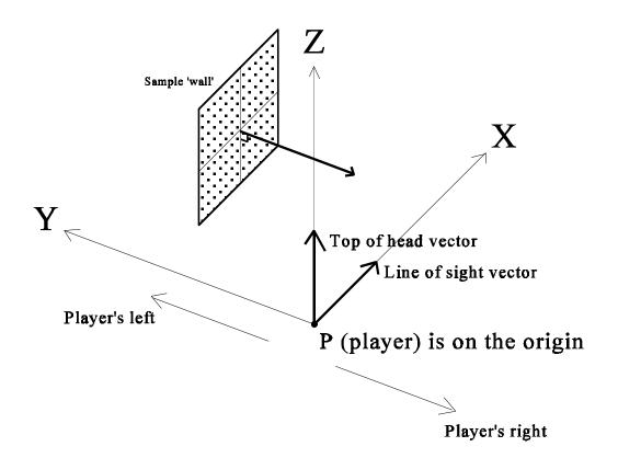
So before using any data for rendering perspective purposes it needs to be translated so P (player) is at the origin. Then rotated so the Line Of Sight vector is collinear with the positive X axis. In my data scheme, I use two points to describe a line in the X/Y plane (novel). Then by associating a Z bottom and a Z top value with it, this line can then represent a 'wall' or polygon in 3-space. That is how all of the walls in my 3D environment are defined.
