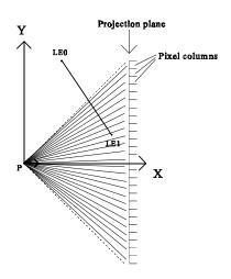
Now you have four linear equations. We know that RayX=WallX and that RayY=WallY so we can easily solve for **t** (which ranges from 0.0 to 1.0). Once you get **t**, multiply it by the width of the wall (128) and you have your horizontal index into the texture. Ideally, you would set the equations up so that **t** would already be scaled by the wall width.
